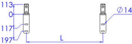
Potelets sans garde-corps | Top fixing without guardrail
